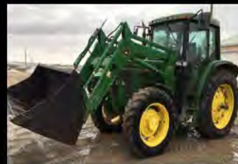
1997 JD 6400 FWA w/ #640 Loader & Duals; 3,006 hrs, LH reverser, hyd center link, 420/80R/38 rears-near new, 13.6-28 fronts, 540/1000 pto, SN# L06400V188708.
